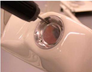
**4.** Remove the tube heads front cover, cable tie and tapes.
