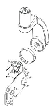
**9.** Place the main cable back to go through the bracket base hole and install the tube head bracket to the handle.
