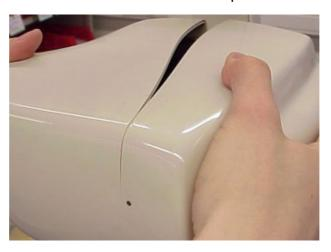
**11.** Fasten the angle ring so that the nodules of the angle ring will meet the hole in the cover. Turn the ring step by step and wedge it with a screwdriver.
