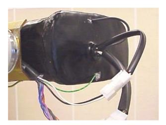
**7.** Remove the screws and locking plates from the bottom of the bracket and remove the tube head.
