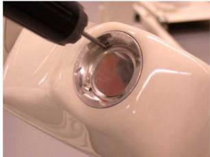
**5.** Remove the tube heads front cover, tapes and the cable tie.
