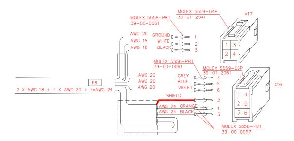
**12.** Check after connecting the X17 connector into it's counterpart that GND wire pins matches.
