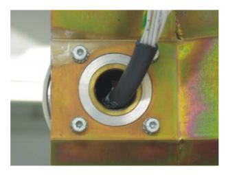
10. Insert the new tube head in to the bracket and remember to set the mylar coat between the tube head and the bracket. Set the locking plates on the bottom of the bracket and tighten the screws with 0.5Nm torgue. Use torgue wrench. Do not use any glues. Fix the locking plates around the bottom screws.
